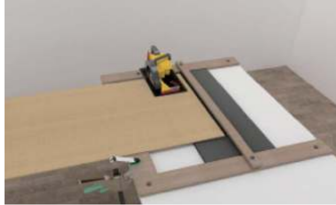
1. Use electric circular saw to cut the wall panel according to the required size.
