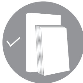
When stacking vertically, provide support and ensure the gap between boards is uniform.
