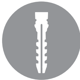
Use plastic sleeve to ensure better grip at the hinges
