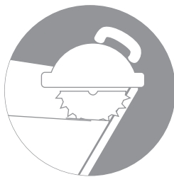
Always cut pre-laminated boards along the scoring line.
