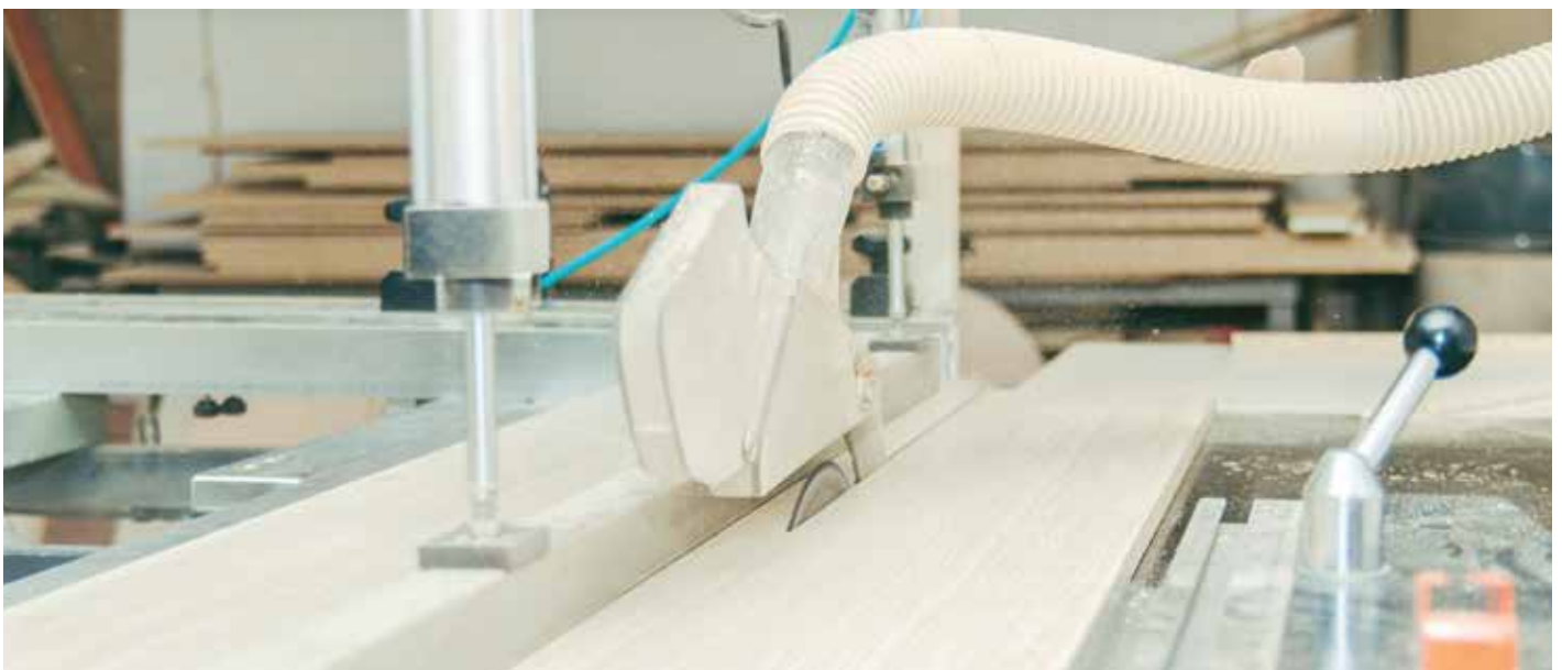
Always cut pre-laminated boards along the scoring line.
