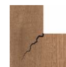
No Claim will be entertained for cracking arising at groove or L-Shape
