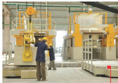
Perfect cutting through 7 Modern Gangsaws
